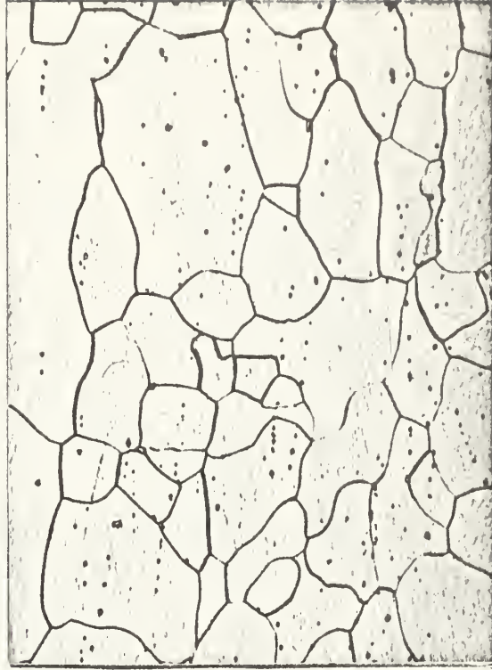
FIG. 22 AT 540°C FOR 30 HOURS (ROCKWELL 30T 33.7)
